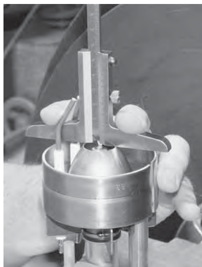
Measurement gap between oil nozzle and air nozzle
